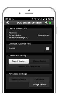
Press the SOS button device for 3 seconds until you hear the buzzer - this way the SOS button will stop being in "sleep" mode. Then, press "Search Devices".
